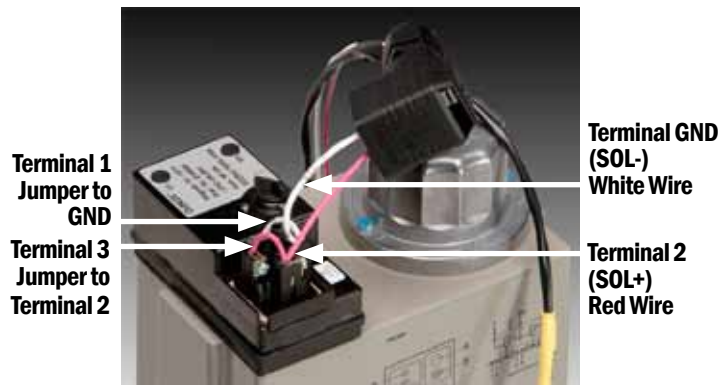
FUEL HARNESS TO ROP CONNECTIONS
