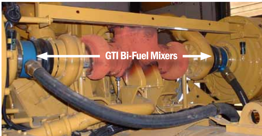
Typical GTI Bi-Fuel System Mixer Installation
